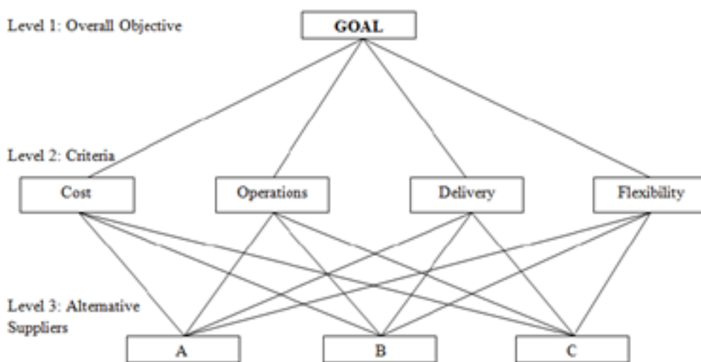
Figure 3. AHP hierarchical structure
