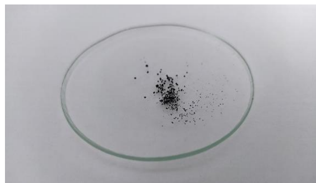
Figure 3. Silver nanoparticles-temu giring rhizome, obtained from freeze-dry
