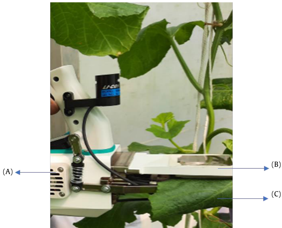
Figure 3. Photosynthetic rate measurement process: (A) LI- 6800 as measuring instrument, (B) chambers LI-6800; (C) melon plant sample leaf
