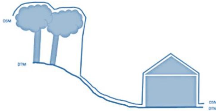
**Figure 2.** Examples of DSM and DTM.
