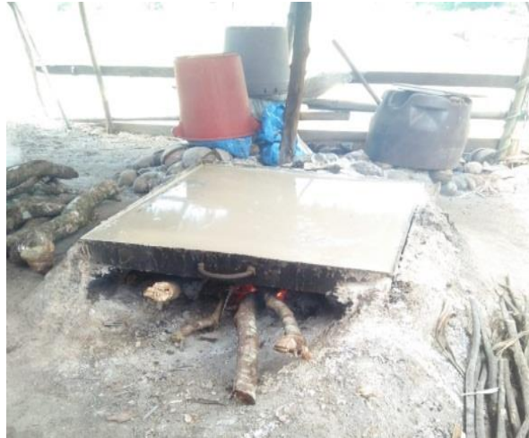
Figure 2. Salt processing using boiling method in East Aceh District.
