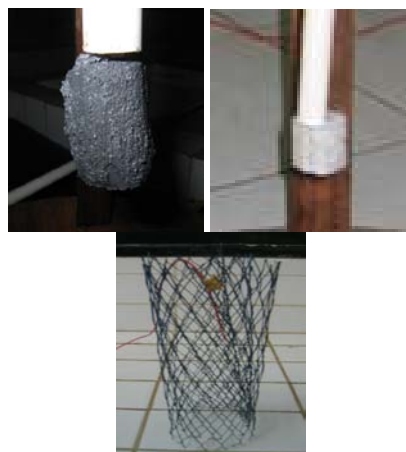
Figure 1. Anode materials used for the Biorock experiment ( left : Aluminum, middle : Magnesium, right : Titanium)
