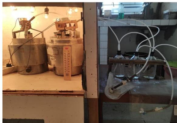
Figure 1. Continuously stirred tank reactor configuration. The biogas digester was placed in the incubator, and the biogas flowed into a bottle filled with NaOH solution and the methane from the bottle was collected using a tedlar gas bag (Oje-Adetule *et al.*, 2023).
